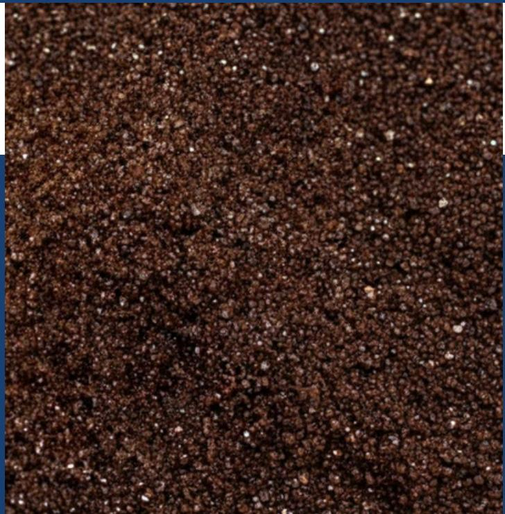
Brown Fused Aluminium Oxide (BFA) is produced by fusing high-quality bauxite in an electric arc furnace at elevated temperatures. The result is a durable abrasive with high hardness, toughness, self-sharpening ability, heat resistance, and chemical stability.
