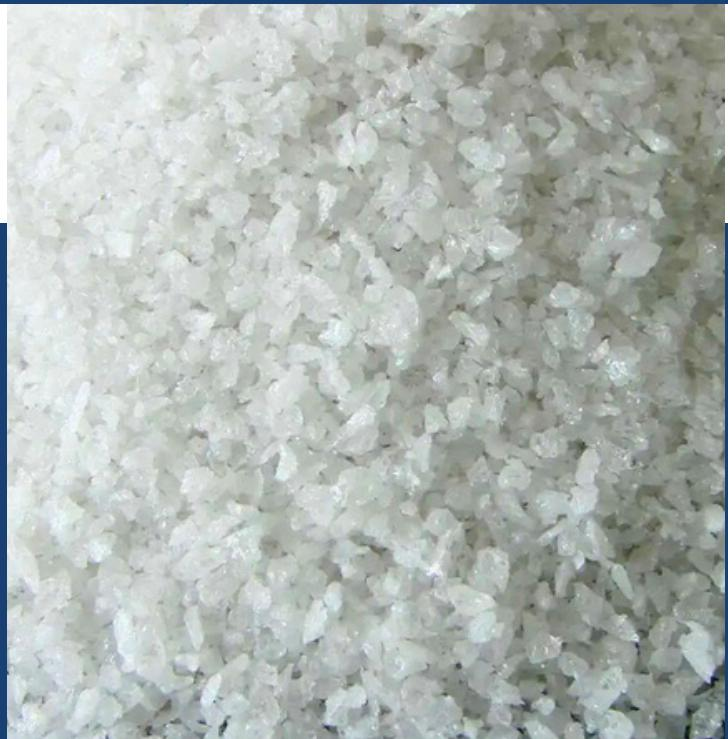
White Aluminum Oxide (White Fused Alumina) is manufactured from imported high-quality alumina, melted above 2000 °C in an electric arc furnace. The result is a pure white abrasive with the main crystal phase  $\alpha\text{-Al}_2\text{O}_3$ .
