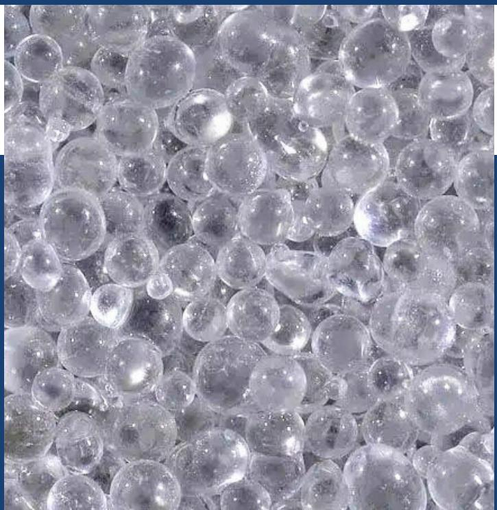
Glass Beads are precision-engineered spherical abrasives manufactured from chemically inert soda-lime glass. Produced from high-grade glass cullet that is melted into spherical form and annealed to equalise internal stresses, they resist fracture and maintain consistent performance.
