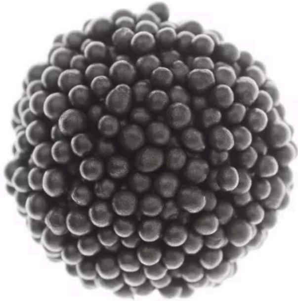
Winoa's steel shot, manufactured under strict conditions and a unique tempering process, allows you to obtain a high carbon cast abrasive shot with optimal resilience, low chlorides & conductivity and high fatigue resistance. Used mainly in shot blasting applications, from desanding in foundries to descaling in steel mills, the HC steel shot will meet your most demanding needs.
